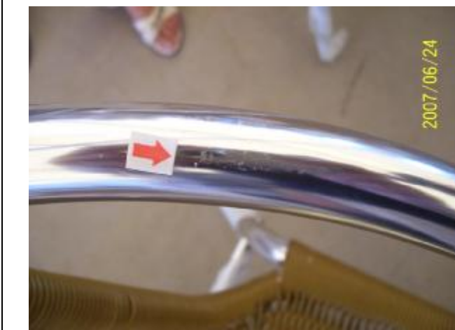
Something jammed at joint: (protect PE sheet)
