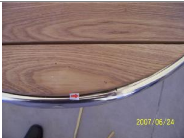
Excessive gap between wood and rim:
