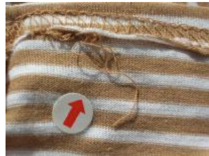
18. minor defect : untrimmed thread end
